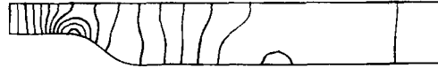
Figure 1(b). Newton–Galerkin incompressible Navier–Stokes algorithm: fine grid, high artificial viscosity coefficient, \lambda = 0.1 , (u^*, p) or PVEC approach
